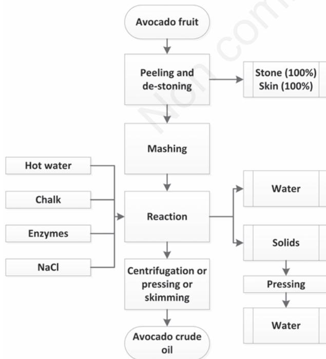
Figure 2. Flow-chart of the traditional mechanical extraction method for avocado oil production.
