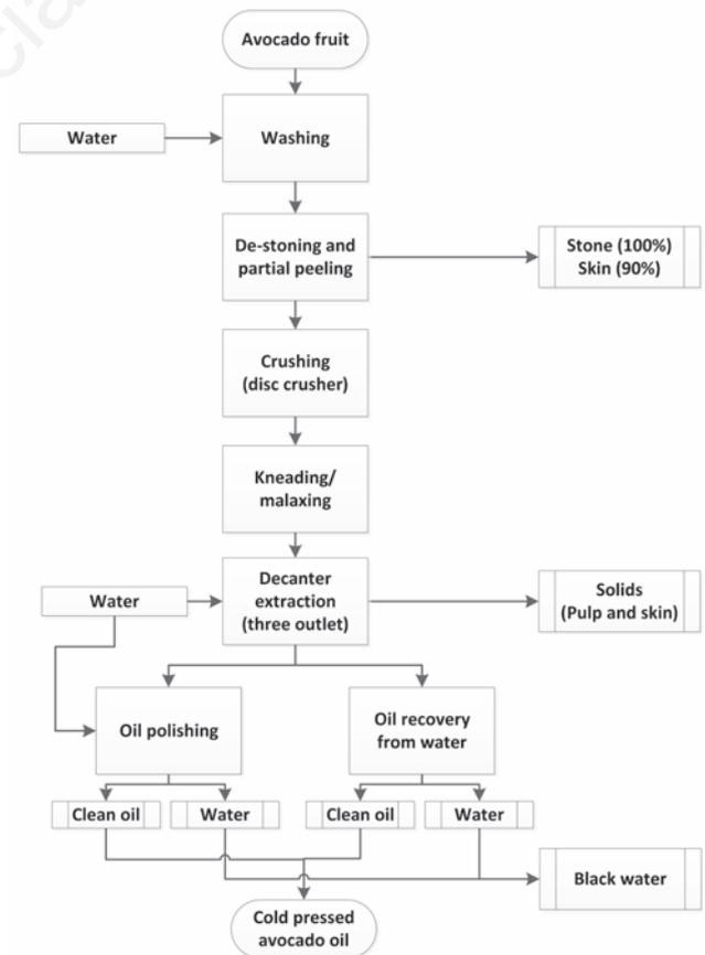
Figure 3. Flow-chart of the cold-pressing mechanical extraction method from Alfa Laval.
