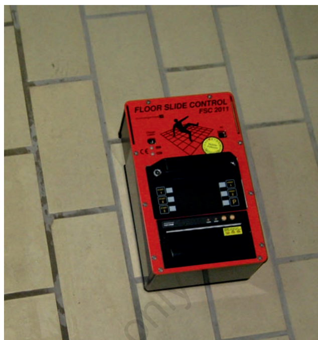
Figure 2. Survey of coefficient of friction on the floor by the Tortus digital tribometer.
