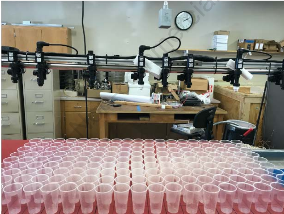
Appendix Figure 2. Experimental testbed for sprayer nozzles.
