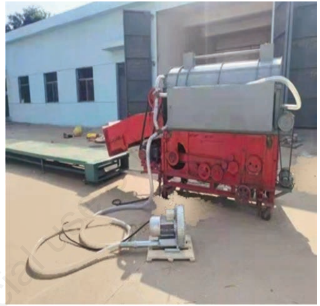
Figure 6. Internal and external drum rotary threshing device.
