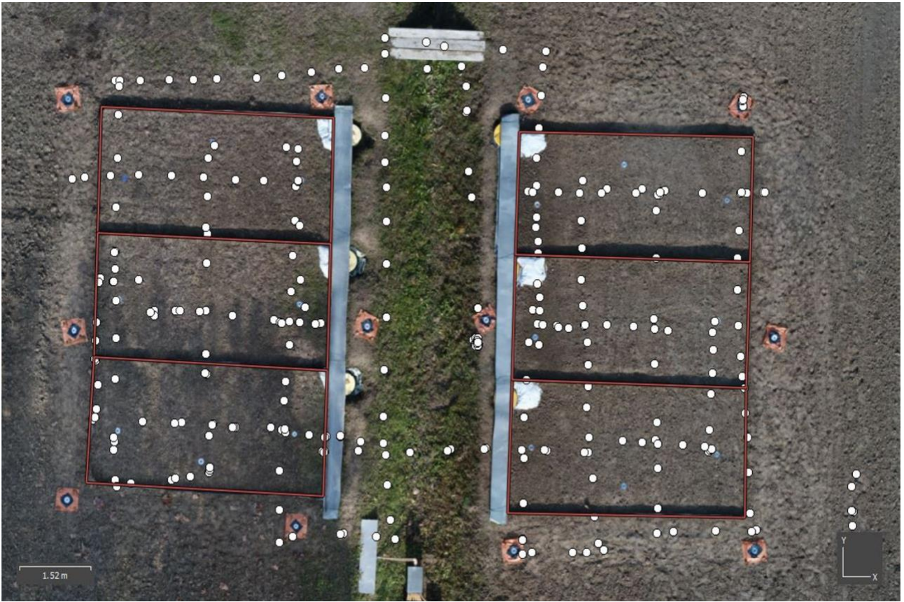
Figure S1. Example of the image network geometry realized for experimental plots. The white circles represent the image position of the SfM survey of November 2019.
