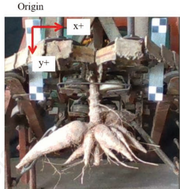
Figure 9. A cassava stalk and the marker on the pulling machine.
