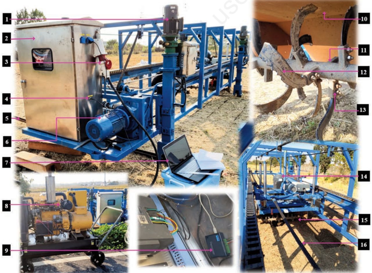
Figure 2. Setup of the test-rig platform: 1- height adjustment motor, 2- control panel, 3- power connection, 4- data cable, 5- rail, 6- traction motor, 7- data acquisition computer, 8- portable generator, 9- Advantech data acquisition module, 10- mudguard, 11- bionic rotary tiller blade, 12- tool holder, 13- rotary shaft motor, 14- assembled experimental rotavator, and 15- drawing chains.
