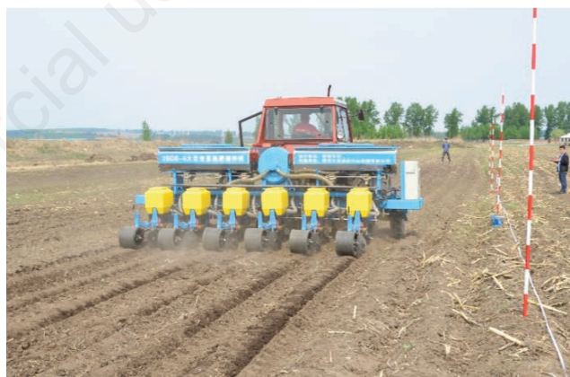
Figure 4. Twin-row planter with subsoiling and experimental plot.
