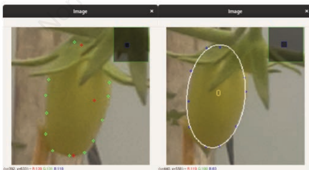
Figure 1. The dots drawn on the edges of the fruit (left) are used to adjust the ellipses (right). The red dots were misplaced and rejected.
