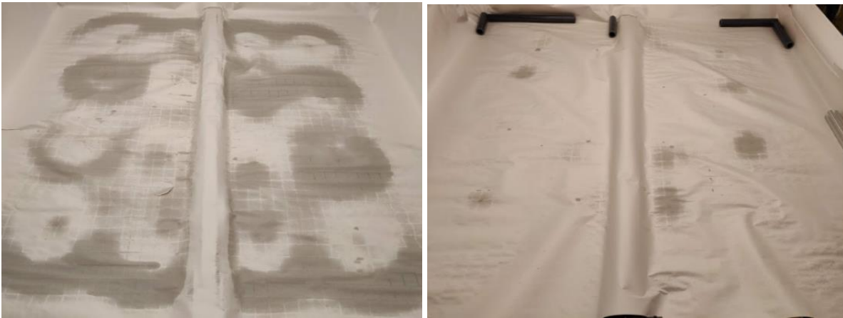
Appendix Figure 8. The spray patterns of the lowest and middle grow tray heights.
