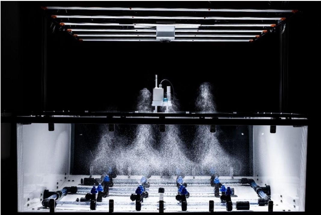
Appendix Figure 7. The spray turns turbulent before reaching the highest grow plane.
