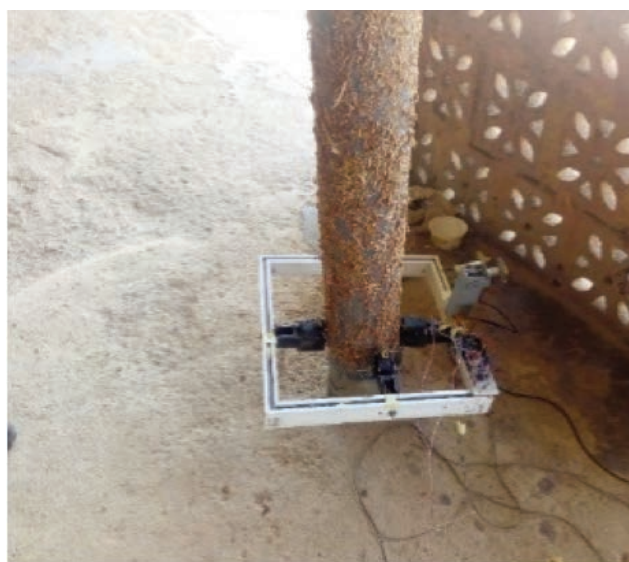
Figure 8. Experimental set-up of Geared DC motor accuracy and Bluetooth module climbing speed test.
