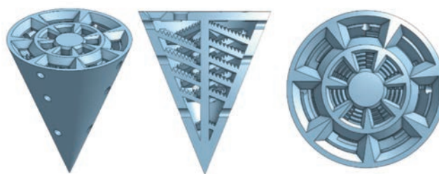
Figure 1. (Left) Rhiome design, (centre) cross-sectional view of Rhiome , (right) top view of Rhiome .
