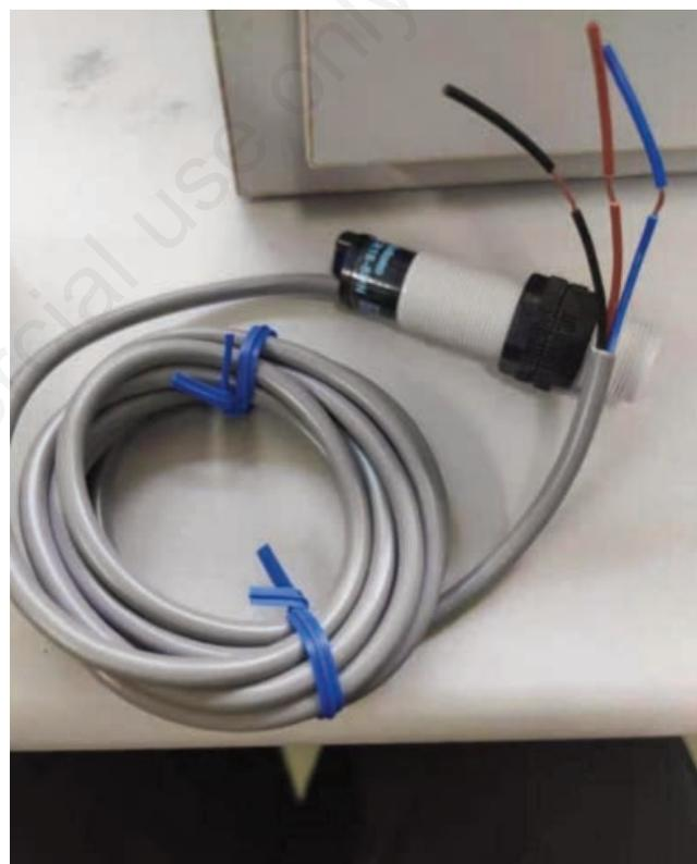
Figure 7. CR18 capacitance sensor.
