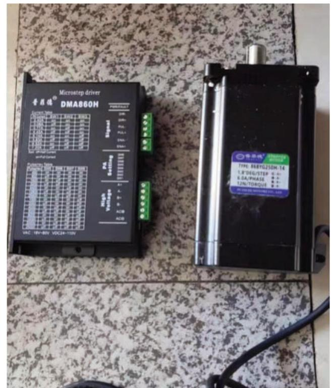
Figure 5. 86BYGH250D stepper motor and HB-860H driver.
