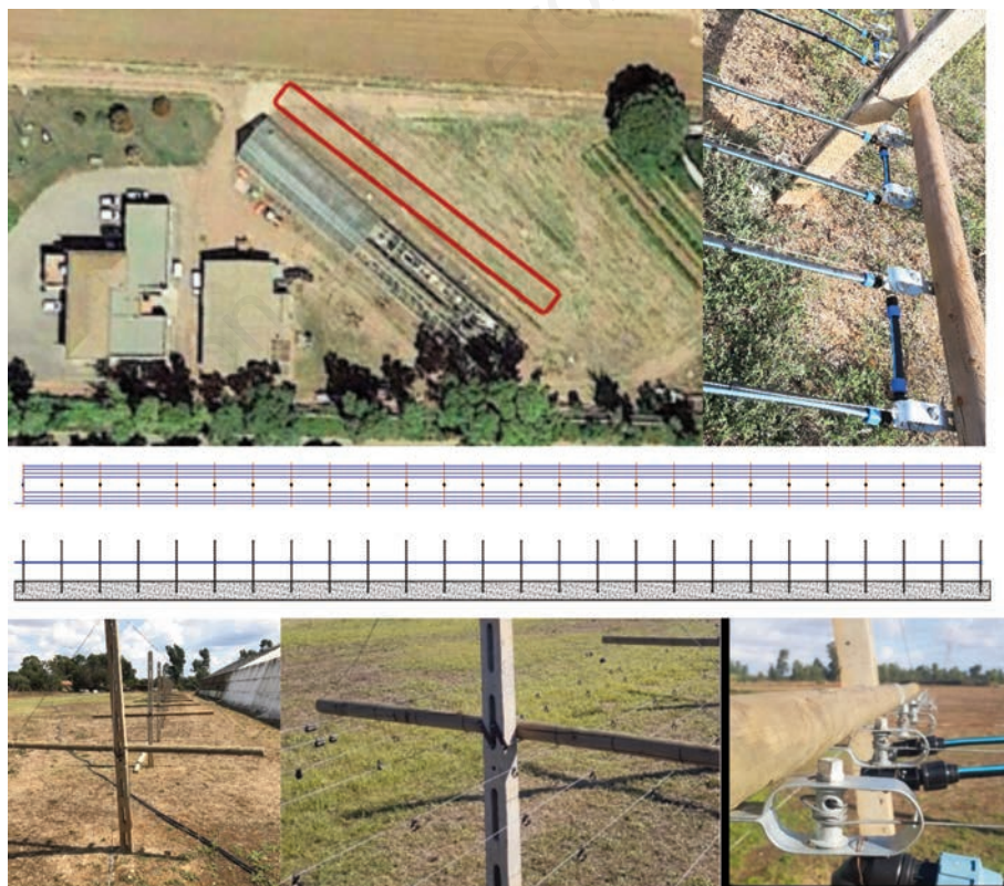
Figure 1. Experimental benchmark layout. Up left: the area occupied by the system. Up right: particular of driplines connection. Centre: system aerial and lateral view. Down left: concrete and wooden poles. Down centre: steel wire for sustaining the dripline. Down right: steel junctions for dripline.
