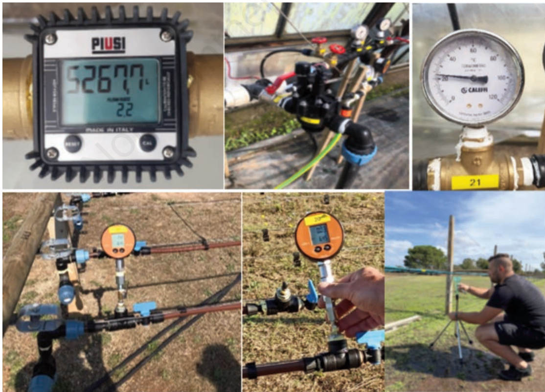
Figure 2. Hydraulic layout particulars. Up left: digital flowmeter. Up centre: pressure head controller. Up right: analogue thermometer. Down left and down centre: example of digital manometers. Down right: example of water collection in the catch can.
