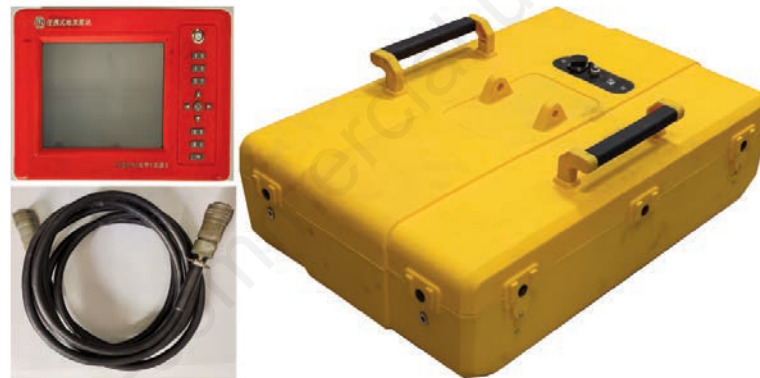
Figure 2. Physical map of detection equipment host, antenna, and data connection line.
