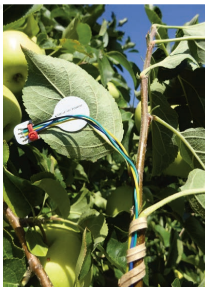
Figure 4. View of the abaxial side of an apple leaf showing the lower side of a capacitance sensor.
