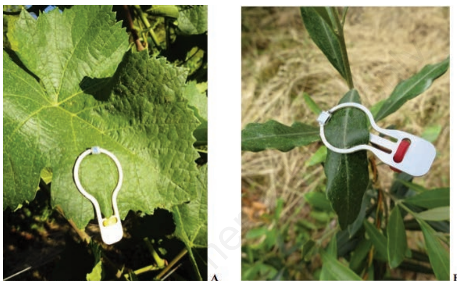
Figure 3. A) Capacitive leaf sensor applied to the grapevine; B) Capacitive leaf sensor applied to the olive.
