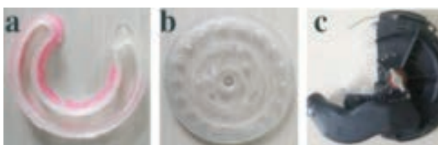
Figure 7. Seeding apparatus parts with transparent treatment. a) Sealed chamber; b) seed disk; c) shell of seeding apparatus.
