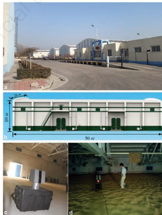
Figure 1. Experimental granary and terrestrial laser scanning data acquisition. (a) A snapshot of Dadushe Grain Reserve depot where experiments took place; (b) front view of the large grain storehouse; (c) scanning experiment under an empty condition; (d) scanning experiment under a full condition.
