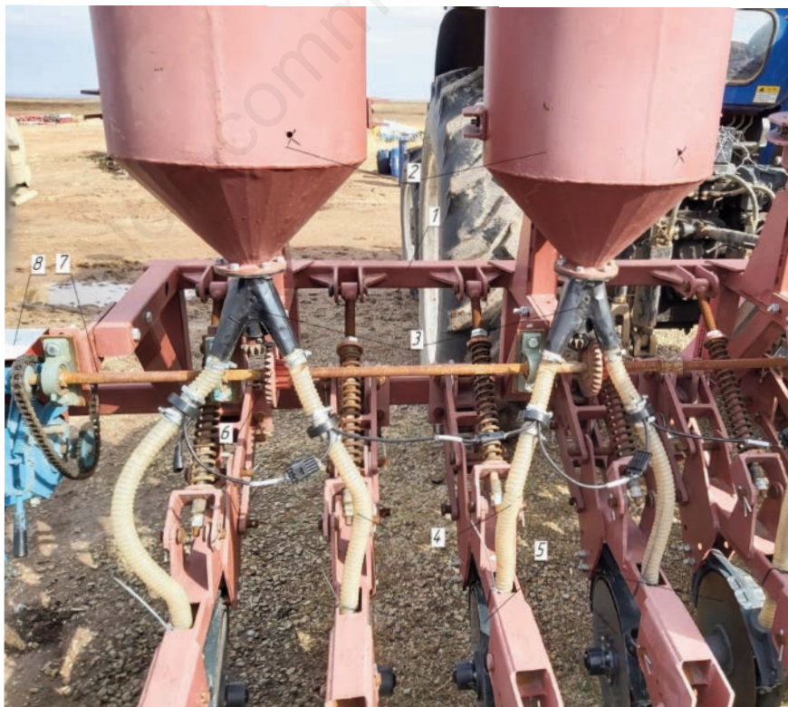
Figure 3. Experimental seeder for sowing non-free-flowing seeds.
