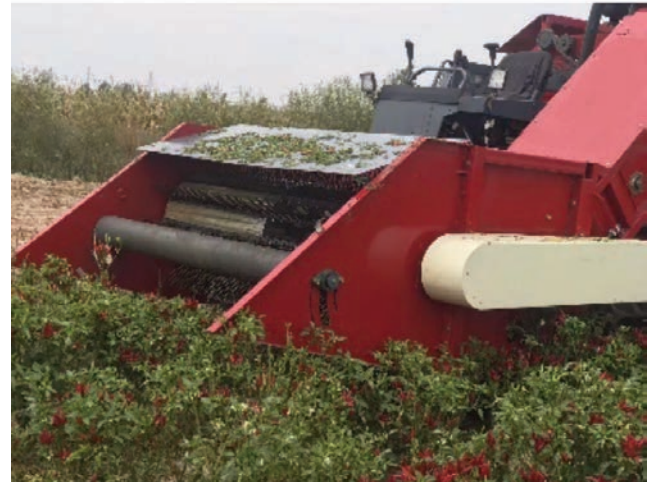
Figure 8. Field test of the prototype picking machine.
