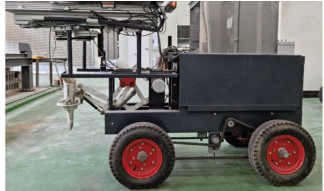
Figure 1. The developed automated vegetable transplanter that requires speed optimization. The transplanter is battery-powered with direct current motors to control its movements.
