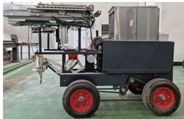
Figure 1. The developed automated vegetable transplanter that requires speed optimization. The transplanter is battery-powered with direct current motors to control its movements.
