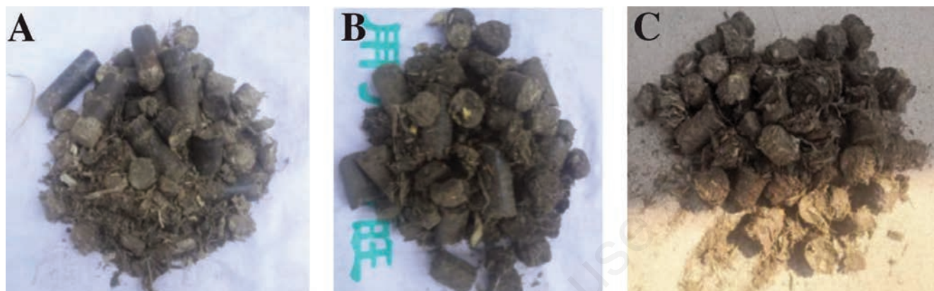
Figure 2. The actual biomass particles. A) low moisture; B) normal moisture; C) high moisture.
