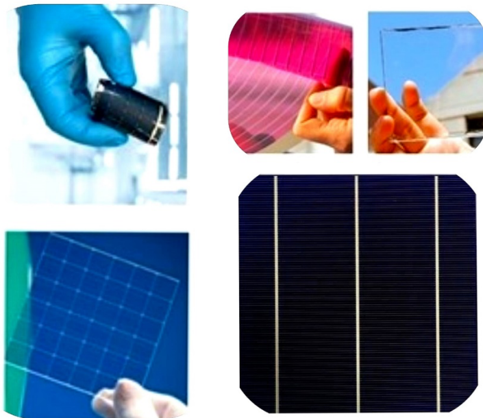
Figure 4. Different PV modules, on the left non selective PV modules, in top right UV-NIR selective cells, and below opaque PV.
