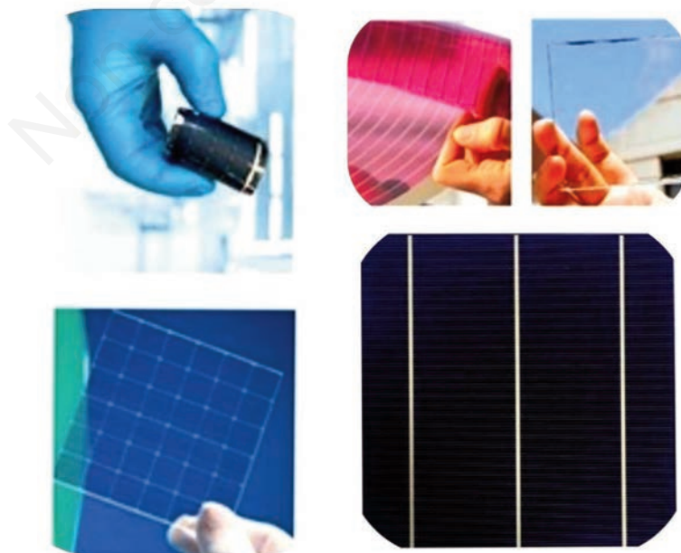
Figure 4. Different PV modules, on the left non selective PV modules, in top right UV-NIR selective cells, and below opaque PV.
