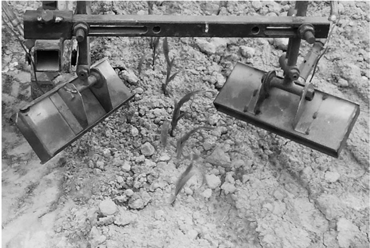
Appendix Figure 3. Cross-flaming application in maize at an early growth stage. Authors acknowledge ASABE as the source of the figure, which is taken from Martelloni et al. , 2016a.
