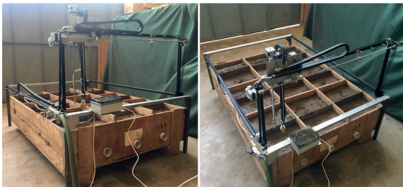
Figure 2. Photographs of the moving bridge manipulator on the soil tank.
