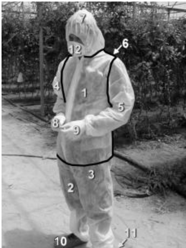
Fig. 4 - Overall to measure the operator dermal exposure.
